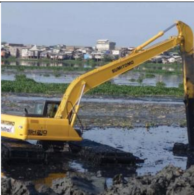
Amphibious excavator AX330ERP upper unit Sumitomo SH210LC-5LR + side undercarriage
